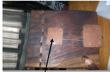
Patched hole where the pickup device was inserted
