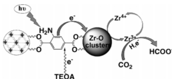
Scheme 1.12: Proposed mechanism for photocatalytic CO 2 reduction over NH 2 -UiO-66(Zr) under visible-light irradiation. 119
