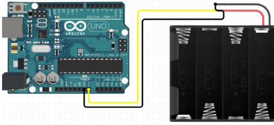
Figure 3.9 Power Supply Unit connected to Arduino Source: Arduino forum 2018
