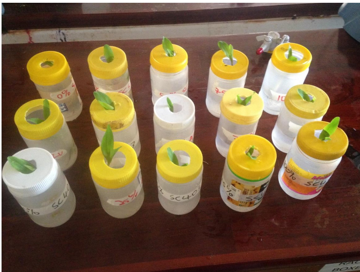
Figure 2: Plastic bottles with different saline concentrations and maize seedling varieties
