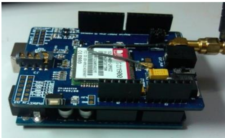
Fig. 3.6 Sim900 GSM/GPRS module mounted onto the Arduino Uno board using the pins and pin holes [#]
