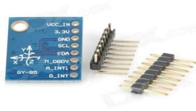
Fig. 2.12 IMU sensor: GY-85 model
