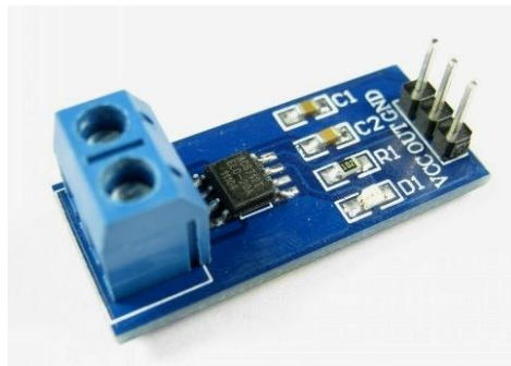
Fig. 2.13 Current Sensor model ACS 712
