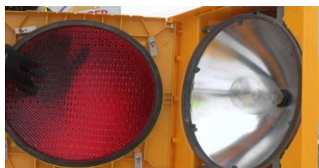
Fig. 2.5 Light bulb traffic signal
