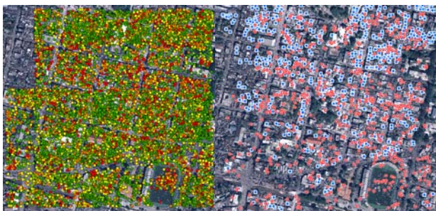
Figure 7 Left: Prediction of collapsed buildings (green = 0-0.4, yellow = 0.4-0.6, orange = 0.6-0.8, red = 0.8-1.0). Right: Image overlaid with reference data (blue) and classified segments (red).
