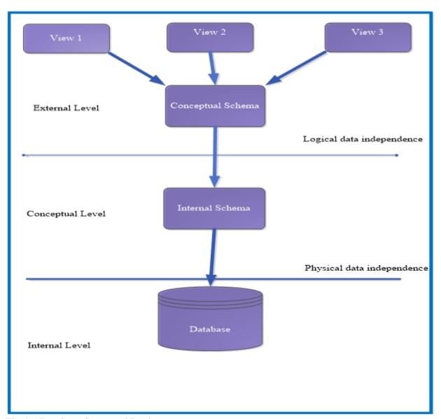
Fig 4.5 Database Structural Design
