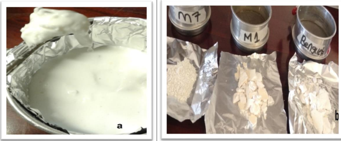
Fig 3.4 a) Starch as a pure white paste before drying; b) powder starch after drying
