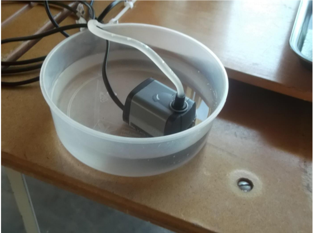
Fig 4.1.1 Water pump and water source
