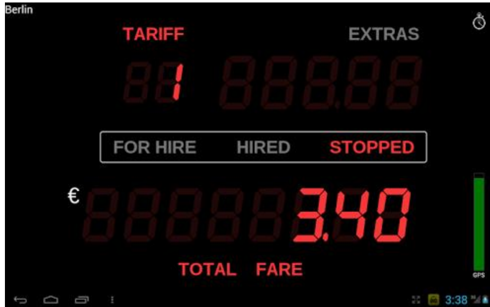
FIGURE: 2.1 An Android™ simulation of modern taximeters
