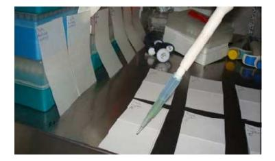
Figure 4: Filter paper impregnation with the acaricide.
