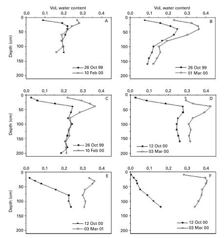
**Figure 5** Wettest and driest water content profiles: (A) sodic bare soil, (B) sodic soil under mopani, (C, D and E) transitional soils that have a duplex character and (F) ridge top site at Mutangi during the 1999/00 and 2000/01 seasons
