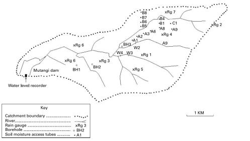
Figure 4 Mutangi instrumentation water level recorder, soil moisture monitoring, boreholes, rain gauges and automatic weather station
