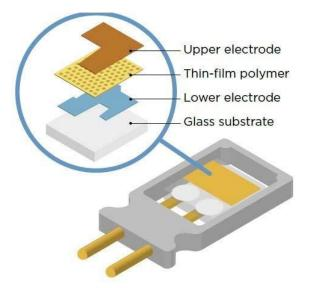
Figure 3. 2: Diagram of a typical Capacitive Humidity Sensor
