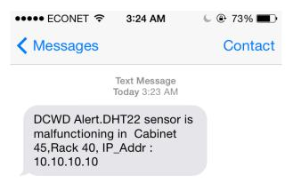
Figure 4. 19: DHT22 malfunction SMS Alert sent by the Data Center Watchdog.
