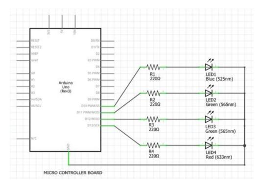
Figure 4. 10: Circuit Diagram of Status LEDs
