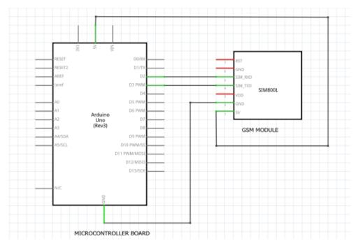
Figure 4. 4 : Connection Schematic of interfacing the SIM800L
