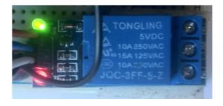
Figure 4. 25: Diagram showing relay state before extreme temperatures were detected.
