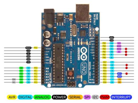
Figure 3. 1: Arduino UNO R3 Pinout Diagram
