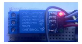
**Figure 4. 26: Diagram showing relay state after extreme temperatures were detected.** Please note that if the green light is off it showing that the relay is in its off state.
