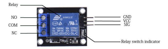
Figure 3. 7: Arduino Single Channel Relay module Pinout Diagram
