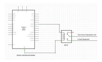
Figure 4. 7: Connection Schematic of interfacing the Relay Module
