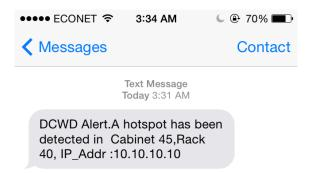
Figure 4. 15: Screenshot of a hotspot SMS alert sent by the Data Center Watchdog.
