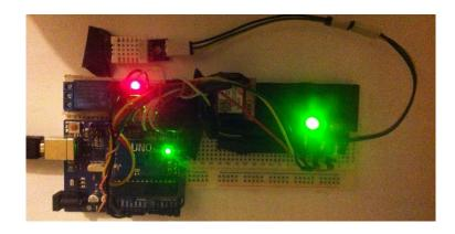
Figure 4. 13: Data Center Watchdog under normal operating mode.
