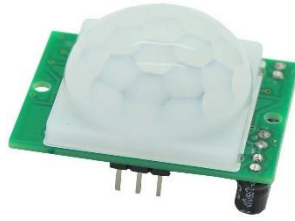
Figure 3.5: Pyroelectric Infrared Motion Sensor (Adapted from Adafruit.com)
