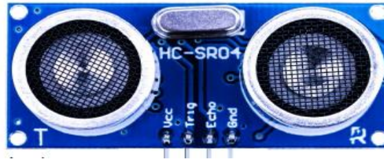
Figure 3.12: Ultrasonic Sensor (Adapted from Adafruit.com)
