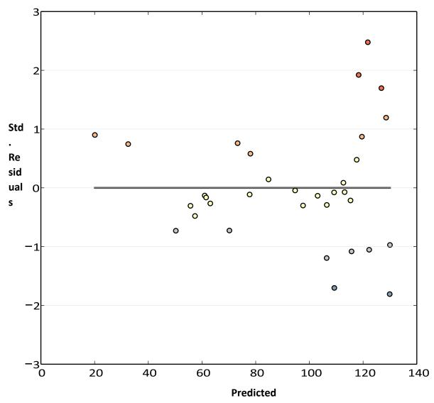
This is a graph of residuals (model over and under predictions) in relation to predicted dependent variable values. For a properly specified model, this scatterplot will have little structure, and look random (see graph on the right). If there is a structure to this plot, the type of structure may be a valuable clue to help you figure out what's going on.
