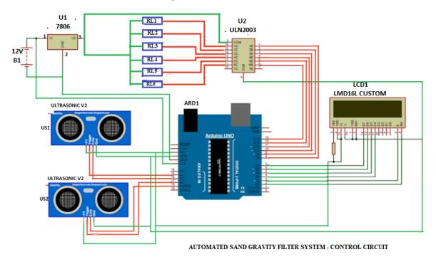
Figure 3.6 – Control circuit schematic for the full system [3]
