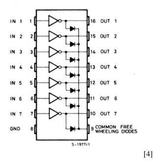
Fig 3.6 – Pin Configuration of a ULN2003 IC
