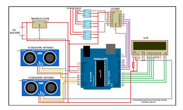
Figure 3.9 – Summarised Control circuit
