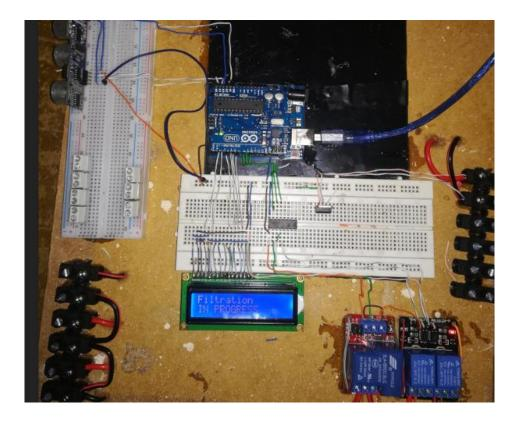
Figure 3.10 – The actual wired control circuit
