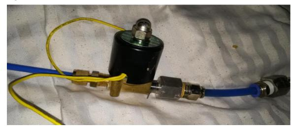
Figure 3.3 – 12Vdc Solenoid valve with connections
