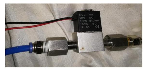
Figure 3.2 - 12Vdc Solenoid Valve with connections
