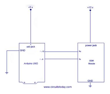
Figure 3.5: Gsm shield to arduino connection
