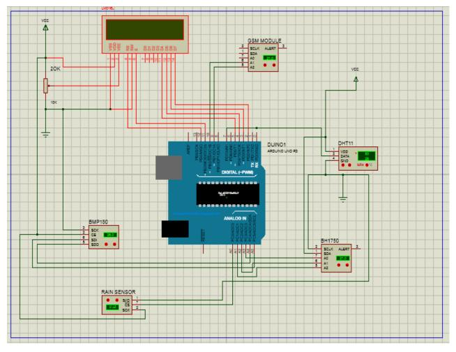
Figure 3.9: System schematic diagram
