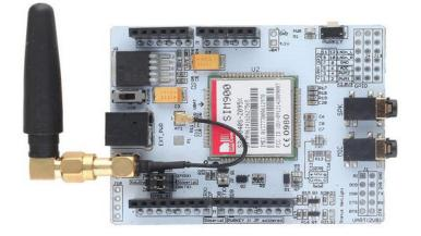
Fig 2.4: Arduino sim900 gprs/gsm shield
