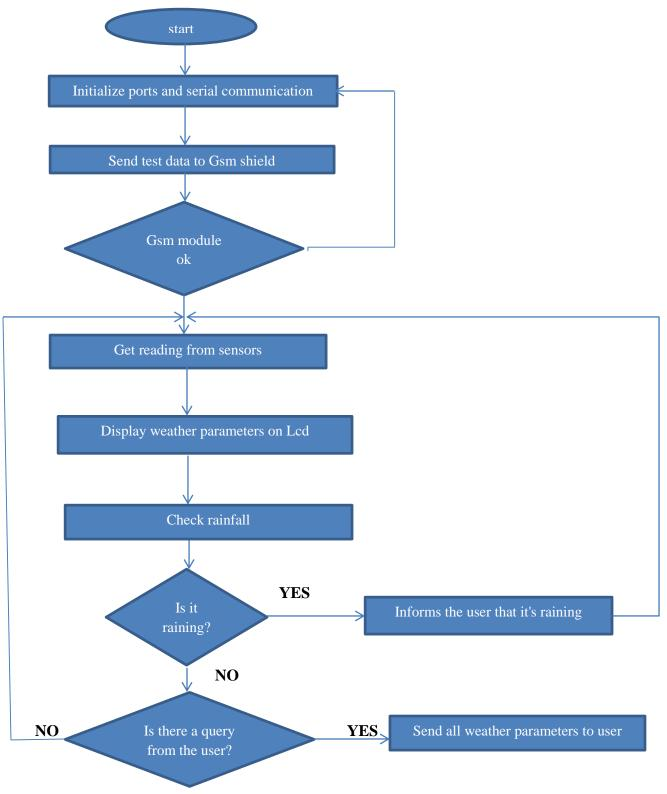
Fig 3.8: system flowchart diagram
