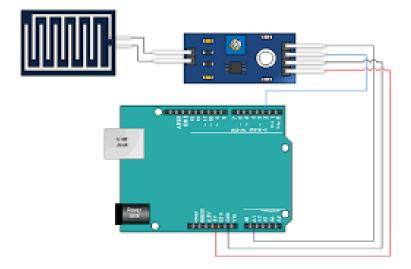
Figure 3.3 below shows raindrop sensor connection with arduino
