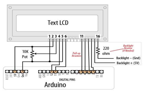
Fig 3.7 : connections for LCD
