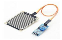
Fig 2.7: raindrop detection sensor
