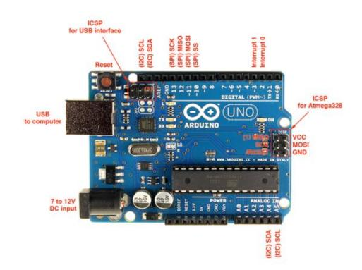
Fig 2.3: Arduino micro-controller board
