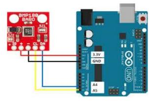
Fig 3.3: BMEP280 connection with arduino
