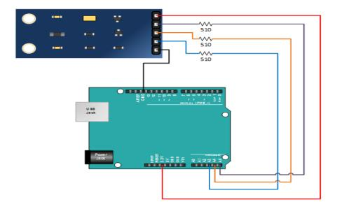
Fig 3.6: BH1750 connection with arduino
