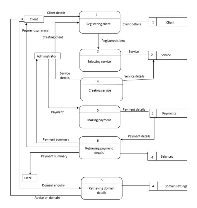
Fig 4.2: Proposed System Data flow diagram
