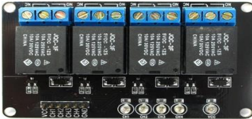
Fig 2.12: 5V 4-Channel Relay Module [17].
