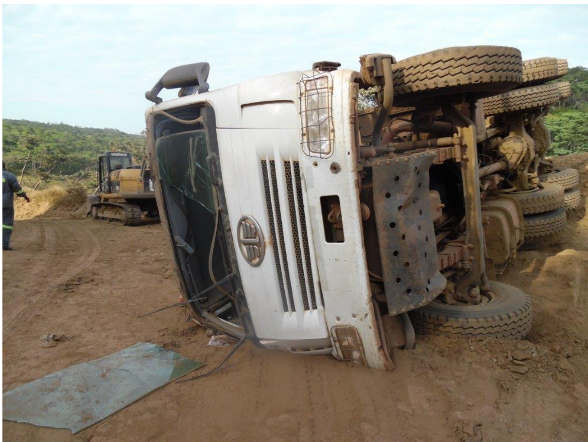
Plate 4.1 Hauling truck fell off on operator’s side at Pit 2 Waste dump.
