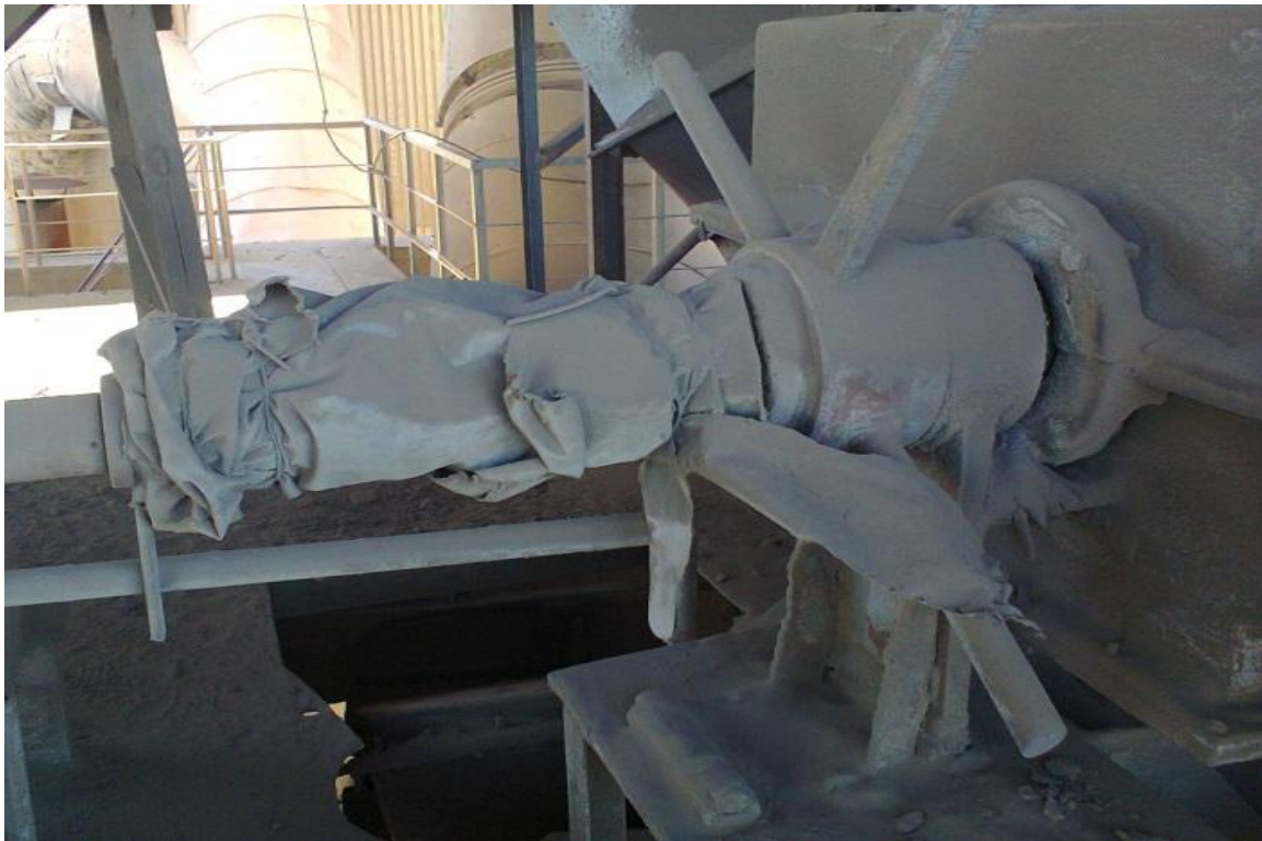
Plate 4.2 An old cement bag used to cover threads of the C5 valve throttle
