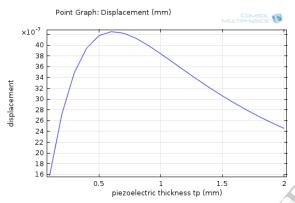
Figure 5. Variation of tip displacement with piezoelectric thickness using structural steel substrate
