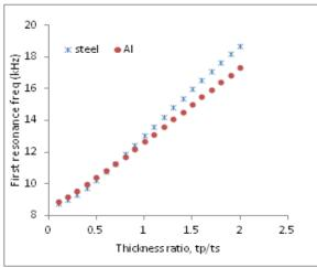
Figure 8. Effect of thickness ratio on first resonance frequency
