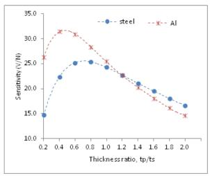
Figure 6. Voltage sensitivity comparison
