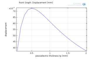
Figure 4. Variation of tip displacement with piezoelectric thickness using aluminium substrate
