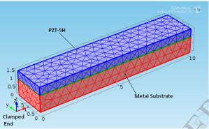
Figure 1. 3D Geometry of unimorph sensor
